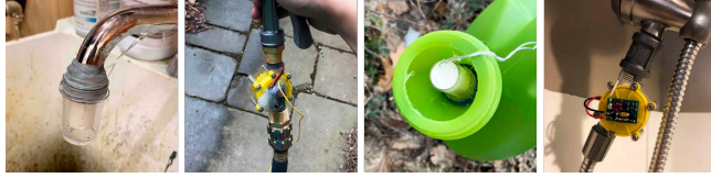
Figure 7. Sozu can be powered by the flow of water from a sink faucet, garden hose, watering can, and showerhead.
