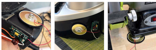
Figure 2. Sozu-augmented objects that convert energy from vibration: sander, blender, and grinding wheel.
