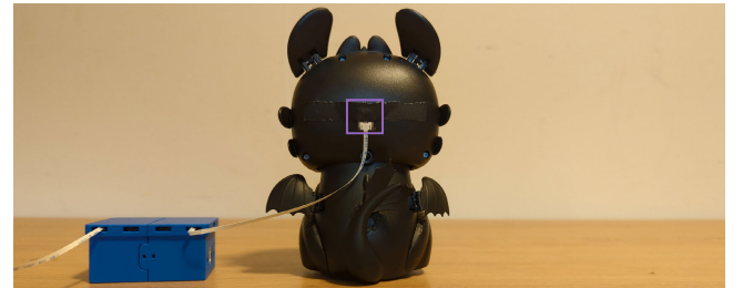
Figure 17: This figure shows how the sensor was affixed to the back of the head of the toy dragon.
