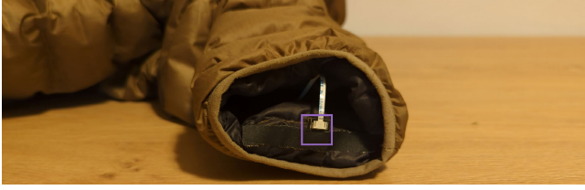
Figure 19: This figure shows how the sensor was affixed to the inside of the jacket sleeve near the cuff.
