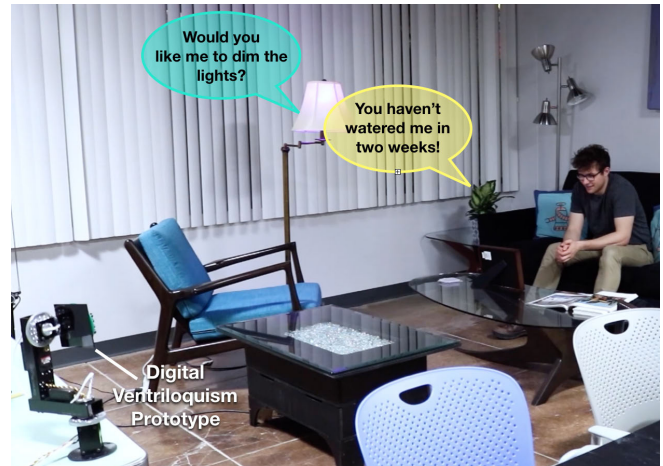
Figure 1. Our system uses a parametric speaker to project ultrasonic beams and render sounds onto passive, everyday objects, appropriating them as interactive voice agents and distributing intelligence throughout environments.
