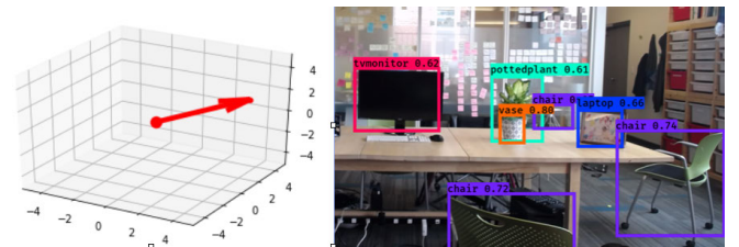
Figure 5. We used a finger snapping interaction and two microphone arrays to capture a 3D vector to an object (left). YOLOv3 provides computer vision recognition and bounding boxes of everyday objects (right).
