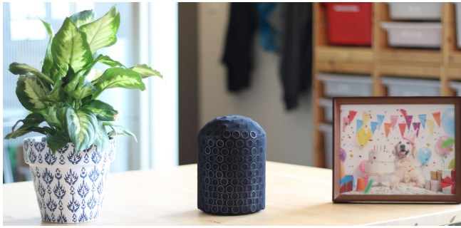
Figure 12. Rather than using a mechanical pan/tilt platform, a future Digital Ventriloquism implementation could utilize a skin of ultrasonic transducers to beamform, as seen in this mockup.
