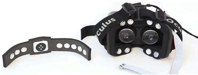
Figure 21. Interferi could be integrated into future smartwatch wristbands and AR/VR headset liners, as seen in these hardware mock-ups.
